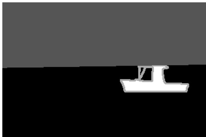
Figure 3.2 Boundaries of foreground objects and pixels outside the ROI are marked by gray value in the ground truth
